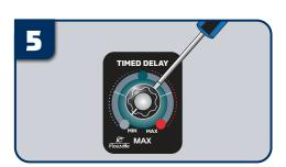
Turn the rotary knob stem all the way to the left (counter-clockwise) until it stops. Place the knob onto the stem with the white indicator pointing to MIN. Tighten the set screw.
